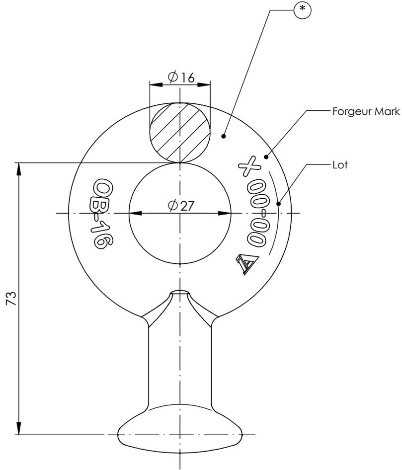
**DIMENSIONS OF BALL ACCORDING TO IEC-60120 N16 STANDARD**
